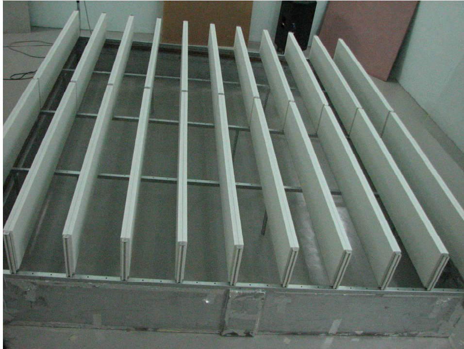
Figure 2 : Aluminum absorption panel setup in reverberation room
