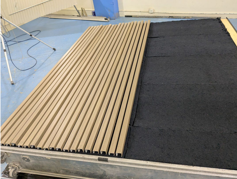
Figure 3 – Specimen pieces partially installed over base layer
