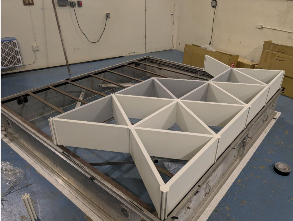
Figure 3 – Specimen grid partially constructed in E-mount frame
