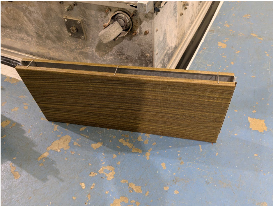
Figure 2 – Individual specimen wall segment
